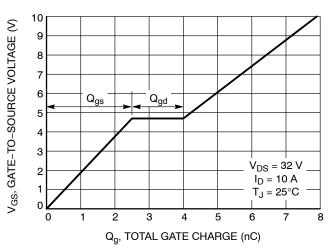
Figure 8. Gate-to-Source Voltage vs. Total Charge
