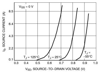
Figure 10. Diode Forward Voltage vs. Current
