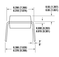
DIMENSIONS: INCHES (MILLIMETERS)  $\frac{\text{MIN}}{\text{MAX}}$
