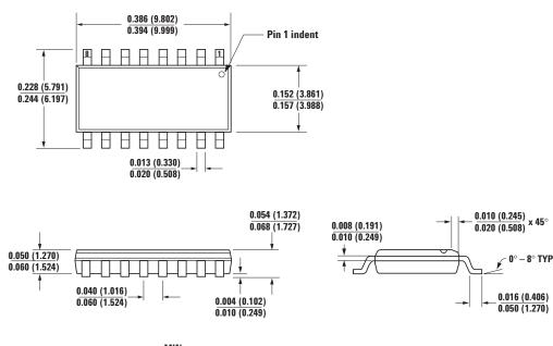
DIMENSIONS: INCHES (MILLIMETERS)  $\frac{\text{MIN}}{\text{MAX}}$
