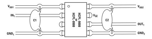
Figure 2. Recommended Printed Circuit Board Layout.
