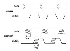
Figure 5. Parallel Data Transmission.
