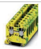
Ground modular terminal block, Connection method: Screw connection, Cross section: 1.5 mm² - 25 mm², AWG: 16 - 4, Width: 12.2 mm, Height: 54.4 mm, Color: green-yellow, Mounting type: NS 35/7,5, NS 35/15
