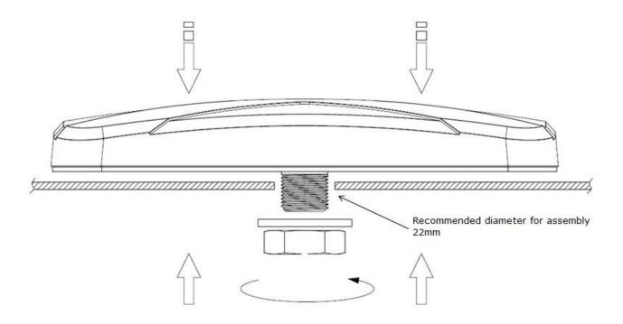
Recommended torque for mounting is 29.4 N.m Maximum torque for mounting is 39.2 N.m
