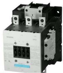
CONTACTOR, 75KW/400V/AC-3, AC(40...60HZ)/DC OPERATION UC 96...127V AUXIL. CONTACTS 2NO+2NC 3-POLE, SIZE S6 BAR CONNECTIONS ELECTRONIC OPERATING MECHANISM WITH PLC INTERFACE 24V DC SCREW TERMINAL
