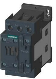
CONTACTOR, AC-3, 11KW/400V, 1NO+1NC, AC110V 50/60HZ, 3-POLE, SZ S0 SCREW TERMINAL
