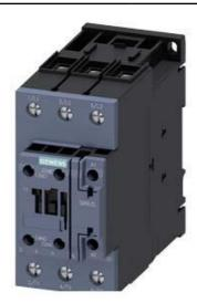
CONTACTOR,AC3:37KW/400V, 1NO+1NC, 230V AC 50HZ, 3-POLE, SIZE S2, SCREW TERMINAL UPRIGHT MOUNTING POSITION
