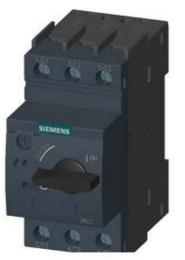
SPECIAL TYPE CIRCUIT BREAKER SIZE S00, FOR TRANSFORMER PROTECTION A-RELEASE 5.5...8A, SHORT-CIRCUIT RELEASE 163A, SCREW TERMINAL, STANDARD SWITCHING CAPACITY AMBIENT TEMPERATURE -50 GRAD 500 SWITCHING CYCLES
