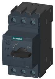
CIRCUIT-BREAKER SZ S00, FOR TRANSFORMER PROT. A-RELEASE 7...10A, N-RELEASE 208A, SCREW CONNECTION, STANDARD SW. CAPACITY
