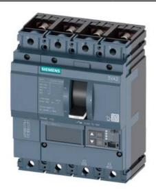
CIRCUIT BREAKER 3VA2 IEC FRAME 100 BREAKING CAPACITY CLASS C ICU=110KA @ 415 V 4POLE, LINE PROTECTION ETU560, LSIG, IN=25A OVERLOAD PROTECTION IR=10A ...25A SHORT CIRCUIT PROTECTION ISD=0,6..10X IN, II=1,5..12X IN NEUTRAL PROTECTION ADJUSTABLE (OFF, UPTO 160%) GROUNDFAULT, SWITCHABLE IG=0,2... 1 X IN, TG=0,050,8MS BUSBAR CONNECTION
