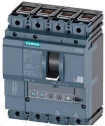
CIRCUIT BREAKER 3VA2 IEC FRAME 100 BREAKING CAPACITY CLASS L ICU=150KA @ 415 V 4POLE, LINE PROTECTION ETU350, LSI, IN=40A OVERLOAD PROTECTION IR=16A ...40A SHORT CIRCUIT PROTECTION ISD=1,5... 10 X IR, II=12 X IN NEUTRAL PROTECTION ADJUSTABLE(OFF,100%) CABLE CONNECTION
