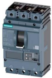
CIRCUIT BREAKER 3VA2 IEC FRAME 160 BREAKING CAPACITY CLASS C ICU=110KA @ 415 V 3POLE, LINE PROTECTION ETU850, LSI, IN=25A OVERLOAD PROTECTION IR=10A ...25A SHORT CIRCUIT PROTECTION ISD=0,6..10X IN, II=1,5..12X IN NEUTRAL PROTECTION OPTIONAL WITH EXT. CT,UPTO 160% BUSBAR CONNECTION
