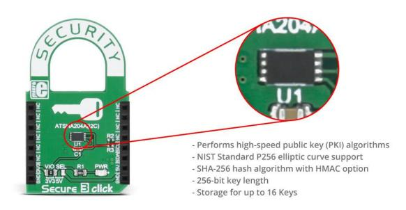
The ATSHA204A device includes an Electrically Erasable Programmable Read-Only Memory (EEPROM) array that can be used for key storage, miscellaneous read/write data, read-only, secret data, consumption logging, and security configuration. Access to the various sections of memory can be restricted in a variety of ways, and the configuration can then be locked to prevent changes.
