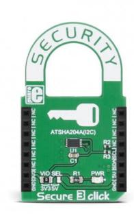
**Secure 3 click** carries the ATSHA204A, a cryptographic coprocessor with secure hardware-based key storage from Microchip. The click is designed to run on either 3.3V or 5V power supply. Secure 3 click communicates with the target microcontroller over an I2C interface. It is ideal to use for:
