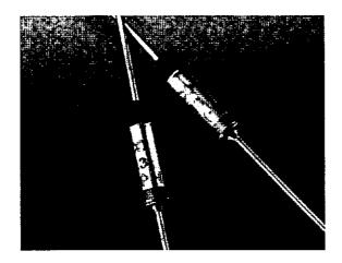
The TCO responds to temperature by interrupting an electrical circuit when the operating and/or environmental temperature exceeds the thermal rating of the fuse. This is accomplished when the organic pellet experiences a phase change, allowing the spring activated contacts to permanently open the circuit.
