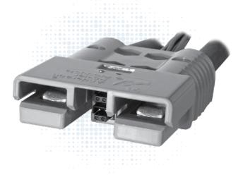
SBX<sup>®</sup> and SBE<sup>®</sup> connectors can integrate up to 8 auxiliary power / signal contacts along with the two primary power circuits. SBE<sup>®</sup> connectors feature an IEC 60950 touch safe housing molded from a chemical resistant PBT/PC blend resin. SBX<sup>®</sup> are molded from a rugged PC resin and are rated IP20 per IEC 60529.
