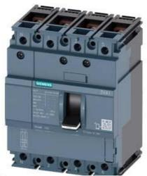
CIRCUIT BREAKER 3VA1 IEC FRAME 100 BREAKING CAPACITY CLASS B ICU=16KA @ 415 V 4-POLE, LINE PROTECTION TM210, FTFM, IN=80A OVERLOAD PROTECTION IR=80A FIXED SHORT CIRCUIT PROTECTION II=10 X IN NEUTRAL UNPROTECTED BUSBAR CONNECTION
