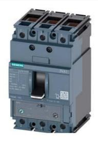
CIRCUIT BREAKER 3VA1 IEC FRAME 160 BREAKING CAPACITY CLASS N ICU=25KA @ 415 V 3-POLE, LINE PROTECTION TM240, ATAM, IN=125A OVERLOAD PROTECTION IR=87,5A ...125A SHORT CIRCUIT PROTECTION II=5...10 X IN CABLE CONNECTION
