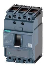
CIRCUIT BREAKER 3VA1 IEC FRAME 160 BREAKING CAPACITY CLASS M ICU=55KA @ 415 V 3-POLE, LINE PROTECTION TM220, ATFM, IN=50A OVERLOAD PROTECTION IR=35A ...50A SHORT CIRCUIT PROTECTION II=10 X IN BUSBAR CONNECTION
