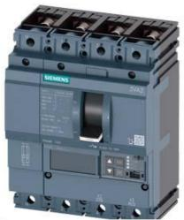
CIRCUIT BREAKER 3VA2 IEC FRAME 100 BREAKING CAPACITY CLASS L ICU=150KA @ 415 V 4POLE, LINE PROTECTION ETU560, LSIG, IN=25A OVERLOAD PROTECTION IR=10A ...25A SHORT CIRCUIT PROTECTION ISD=0,6..10X IN, II=1,5..12X IN NEUTRAL PROTECTION ADJUSTABLE (OFF, UPTO 160%) GROUNDFAULT, SWITCHABLE IG=0,2... 1 X IN, TG=0,050,8MS BUSBAR CONNECTION
