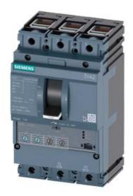
CIRCUIT BREAKER 3VA2 IEC FRAME 100 BREAKING CAPACITY CLASS C ICU=110KA @ 415 V 3POLE, LINE PROTECTION ETU350, LSI, IN=40A OVERLOAD PROTECTION IR=16A ...40A SHORT CIRCUIT PROTECTION ISD=1,5... 10 X IR, II=12 X IN CABLE CONNECTION
