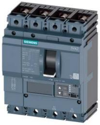
CIRCUIT BREAKER 3VA2 IEC FRAME 160 BREAKING CAPACITY CLASS L ICU=150KA @ 415 V 4POLE, LINE PROTECTION ETU550, LSI, IN=25A OVERLOAD PROTECTION IR=10A ...25A SHORT CIRCUIT PROTECTION ISD=0,6..10X IN, II=1,5..12X IN NEUTRAL PROTECTION ADJUSTABLE (OFF, UPTO 160%) BUSBAR CONNECTION
