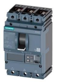
CIRCUIT BREAKER 3VA2 IEC FRAME 250 BREAKING CAPACITY CLASS M ICU=55KA @ 415 V 3POLE, LINE PROTECTION ETU850, LSI, IN=250A OVERLOAD PROTECTION IR=100A ...250A SHORT CIRCUIT PROTECTION ISD=0,6..10X IN, II=1,5..10X IN NEUTRAL PROTECTION OPTIONAL WITH EXT. CT,UPTO 160% BUSBAR CONNECTION
