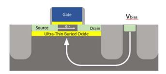
**Body Biasing**: Faster when required and more energy efficient when performance isn't as critical
