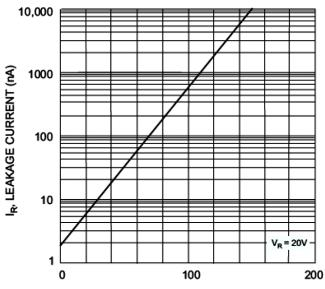
T<sub>j</sub>, JUNCTION TEMPERATURE (°C) Fig. 2 Leakage Current vs Junction Temperature
