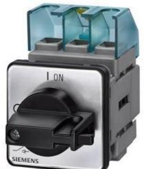
MAIN CONTROL SWITCH 3-POLE IU=32, P/AC-23A AT 400V=11,5KW FRONT MOUNTING CENTRAL-HOLE MOUNTING KNOB BLACK
