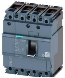
CIRCUIT BREAKER 3VA1 IEC FRAME 160 BREAKING CAPACITY CLASS N ICU=25KA @ 415 V 4-POLE, LINE PROTECTION TM210, FTFM, IN=125A OVERLOAD PROTECTION IR=125A FIXED SHORT CIRCUIT PROTECTION II=10 X IN NEUTRAL UNPROTECTED BUSBAR CONNECTION
