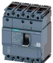
CIRCUIT BREAKER 3VA1 IEC FRAME 160 BREAKING CAPACITY CLASS H ICU=70KA @ 415 V 4-POLE, LINE PROTECTION TM210, FTFM, IN=20A OVERLOAD PROTECTION IR=20A FIXED SHORT CIRCUIT PROTECTION II=10 X IN NEUTRAL PROTECTION 100% BUSBAR CONNECTION
