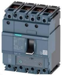
CIRCUIT BREAKER 3VA1 IEC FRAME 160 BREAKING CAPACITY CLASS H ICU=70KA @ 415 V 4-POLE, LINE PROTECTION TM240, ATAM, IN=32A OVERLOAD PROTECTION IR=22,4A ...32A SHORT CIRCUIT PROTECTION II=5...10 X IN NEUTRAL UNPROTECTED BUSBAR CONNECTION
