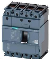
CIRCUIT BREAKER 3VA1 IEC FRAME 160 BREAKING CAPACITY CLASS N ICU=25KA @ 415 V 4-POLE, LINE PROTECTION TM210, FTFM, IN=50A OVERLOAD PROTECTION IR=50A FIXED SHORT CIRCUIT PROTECTION II=10 X IN NEUTRAL PROTECTION 100% CABLE CONNECTION
