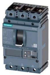
CIRCUIT BREAKER 3VA2 IEC FRAME 100 BREAKING CAPACITY CLASS C ICU=110KA @ 415 V 3POLE, LINE PROTECTION ETU850, LSI, IN=40A OVERLOAD PROTECTION IR=16A ...40A SHORT CIRCUIT PROTECTION ISD=0,6..10X IN, II=1,5..12X IN NEUTRAL PROTECTION OPTIONAL WITH EXT. CT,UPTO 160% BUSBAR CONNECTION
