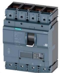
CIRCUIT BREAKER 3VA2 IEC FRAME 400 BREAKING CAPACITY CLASS H ICU=85KA @ 415 V 4-POLE, LINE PROTECTION ETU560, LSIG, IN=400A OVERLOAD PROTECTION IR=160A ...400A SHORT CIRCUIT PROTECTION ISD=0,6..10X IN, II=1,5..10X IN NEUTRAL PROTECTION ADJUSTABLE (OFF, UPTO 100%) GROUND-FAULT, SWITCHABLE IG=0,2... 1 X IN, TG=0,05-0,8MS BUSBAR CONNECTION
