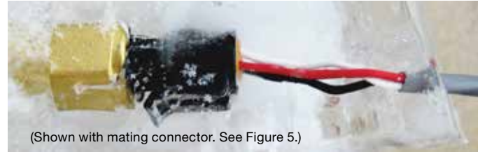
Figure 2. PX3 Series External Freeze/Thaw Resistance
