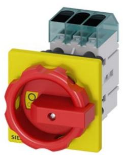
Load disconnector 3LD3, Iu 40 A Main switch 3-pole Rated operating capacity at AC-23 A at 400 V 15.0 kW Front plate mounting Basic switch with Central hole mounting 22.5mm Toggle drive red / yellow 66x66 mm
