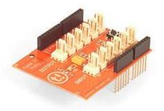
**Module description**: A green LED signals that the shield is correctly powered, a standard 6mm pushbutton allows you to RESET the board.
