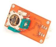
**Module Description**: This module features two 4k7 Ohm linear potentiometers, two standard TinkerKit 3pin connector, two signal amplifiers, a green LED that signals that the module is correctly powered and two yellow LED whose brightness depends on the values output by the module.
