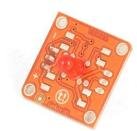
This module is an **ACTUATOR** therefore the connector is an INPUT that need to be connected to one of the **OUTPUT** connectors on the **TinkerKit Shield**.
