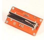
**Module Description**: this module features a 4k7 Ohm linear potentiometer, a signal amplifier, the standard TinkerKit 3pin connector, a green LED that signals that the module is correctly powered and a yellow LED whose brightness changes according to the position of the potentiometer.
