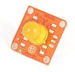
**Module description**: this module features a 10mm Yellow Light Emitting Diode, the standard TinkerKit 3pin connector and a green LED that signals that the module is correctly powered and a tiny yellow LED that shows the current brightness of the yellow LED. A resistor provides the optimal amount of current when connected to an Arduino.
