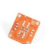
The **Tilt Sensor** can detect when it is at an angle.
