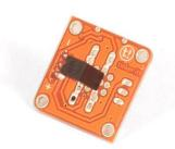
**Module description**: this module features a Tilt Sensor, a signal amplifier, the standard TinkerKit 3pin connector, a green LED that signals that the module is correctly powered and a yellow LED that lights up when a connection is made (the sensor is upright).
