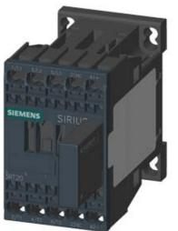
COUPLING RELAY, AC-3, 3KW/400V, 1NC, DC 24V, 0.85...1.85\*US, W. PLUGGED-ON VARISTOR 3-POLE SZ S00, SPRING-LOADED TERMINAL
