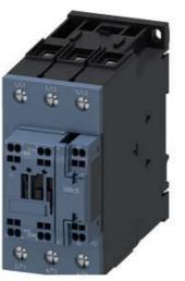
CONTACTOR,AC3:37KW/400V, 1NO+1NC, 20-33VAC/DC, COM.CAP. WITH VARISTOR, 3-POLE, SIZE S2, SPRING-TYPE TERMINAL
