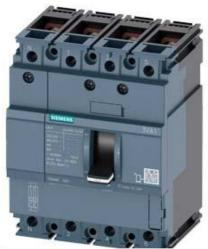
CIRCUIT BREAKER 3VA1 IEC FRAME 160 BREAKING CAPACITY CLASS M ICU=55KA @ 415 V 4-POLE, LINE PROTECTION TM210, FTFM, IN=100A OVERLOAD PROTECTION IR=100A FIXED SHORT CIRCUIT PROTECTION II=10 X IN NEUTRAL PROTECTION 100% BUSBAR CONNECTION
