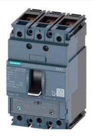
CIRCUIT BREAKER 3VA1 IEC FRAME 160 BREAKING CAPACITY CLASS H ICU=70KA @ 415 V 3-POLE, LINE PROTECTION TM240, ATAM, IN=40A OVERLOAD PROTECTION IR=28A ...40A SHORT CIRCUIT PROTECTION II=5...10 X IN BUSBAR CONNECTION
