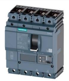
CIRCUIT BREAKER 3VA2 IEC FRAME 100 BREAKING CAPACITY CLASS M ICU=55KA @ 415 V 4POLE, LINE PROTECTION ETU560, LSIG, IN=63A OVERLOAD PROTECTION IR=25A ...63A SHORT CIRCUIT PROTECTION ISD=0,6..10X IN, II=1,5..12X IN NEUTRAL PROTECTION ADJUSTABLE (OFF, UPTO 160%) GROUNDFAULT, SWITCHABLE IG=0,2... 1 X IN, TG=0,050,8MS BUSBAR CONNECTION
