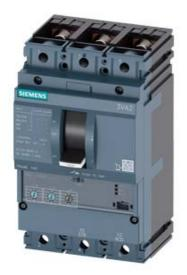
CIRCUIT BREAKER 3VA2 IEC FRAME 160 BREAKING CAPACITY CLASS L ICU=150KA @ 415 V 3POLE, LINE PROTECTION ETU320, LI, IN=25A OVERLOAD PROTECTION IR=10A ...25A SHORT CIRCUIT PROTECTION II=12 X IN BUSBAR CONNECTION
