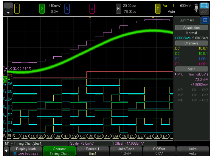
Figure 26. Analog and digital signals displayed together with the logic timing chart function.
