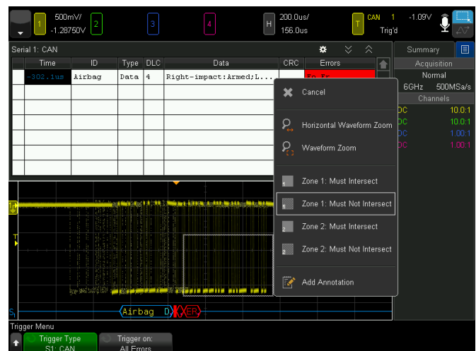
Figure 13. Setting up the zone trigger in addition to a CAN bus error packet trigger.
