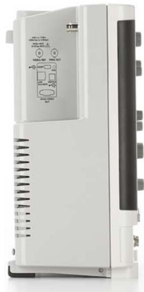
Figure 8. One- gigahertz-per-inch form factor: 6 GHz, 6 inches deep.
