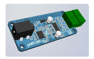
pHAT-HIFI is a high fidelity 32bit stereo DAC audio module with a high efficiency 12+12Watt Class-D power amplifier to drive 4 or  $8\Omega$  speakers. Specifically designed for the Raspberry-Pi Zero user (can also be used on all the other Raspberry-Pi variants) the pHAT-HIFI features 32bit 3 wire I<sup>2</sup>S (PCM) communication to reproduce low noise, high quality audio in any voice or music application.
