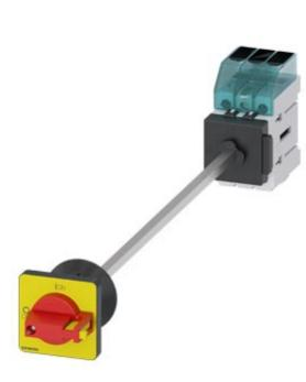
Switch disconnector 3LD3, main switch 3-polig, lu 16A operational switch at AC-23 A at 400 V 7,5 kW floor mounting Base mounting with door coupling center-hole 22,5 mm knob-operated mechanism red/yellow 48 x 48 mm
