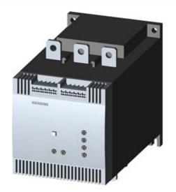
SIRIUS SOFT STARTER, S12, 205 A, 150 HP/460 V, 50 DEG., 200-460 V AC, 115 V AC, CAGE CLAMP TERMINALS
