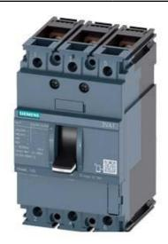
CIRCUIT BREAKER 3VA1 IEC FRAME 100 BREAKING CAPACITY CLASS B ICU=16KA @ 415 V 3-POLE, LINE PROTECTION TM210, FTFM, IN=16A OVERLOAD PROTECTION IR=16A FIXED SHORT CIRCUIT PROTECTION II=10 X IN BUSBAR CONNECTION
