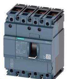
CIRCUIT BREAKER 3VA1 IEC FRAME 160 BREAKING CAPACITY CLASS N ICU=25KA @ 415 V 4-POLE, LINE PROTECTION TM210, FTFM, IN=50A OVERLOAD PROTECTION IR=50A FIXED SHORT CIRCUIT PROTECTION II=10 X IN NEUTRAL PROTECTION 100% BUSBAR CONNECTION
