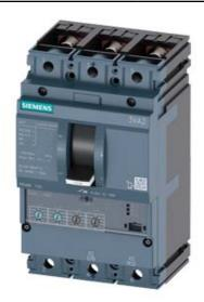
CIRCUIT BREAKER 3VA2 IEC FRAME 100 BREAKING CAPACITY CLASS H ICU=85KA @ 415 V 3POLE, LINE PROTECTION ETU330, LIG, IN=40A OVERLOAD PROTECTION IR=16A ...40A SHORT CIRCUIT PROTECTION II=1,5...12 X IN GROUNDFAULTPROTECTION IG=0,2... 1 X IN, TG=0,1/0,3MS BUSBAR CONNECTION
