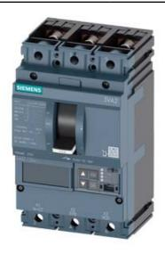
CIRCUIT BREAKER 3VA2 IEC FRAME 250 BREAKING CAPACITY CLASS L ICU=150KA @ 415 V 3POLE, LINE PROTECTION ETU560, LSIG, IN=160A OVERLOAD PROTECTION IR=64A ...160A SHORT CIRCUIT PROTECTION ISD=0,6..10X IN, II=1,5..12X IN NEUTRAL PROTECTION OPTIONAL WITH EXT. CT,UPTO 160% GROUNDFAULT, SWITCHABLE IG=0,2... 1 X IN, TG=0,050,8MS BUSBAR CONNECTION
