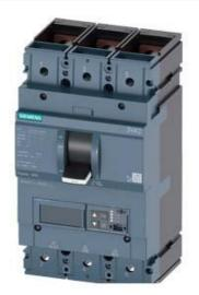
CIRCUIT BREAKER 3VA2 IEC FRAME 400 BREAKING CAPACITY CLASS C ICU=110KA @ 415 V 3-POLE, LINE PROTECTION ETU860, LSIG, IN=250A OVERLOAD PROTECTION IR=100A ...250A SHORT CIRCUIT PROTECTION ISD=0,6..10X IN, II=1,5..12X IN NEUTRAL PROTECTION OPTIONAL WITH EXT. CT;UPTO 160% GROUND-FAULT, SWITCHABLE IG=0,2... 1 X IN, TG=0,05-0,8MS BUSBAR CONNECTION
