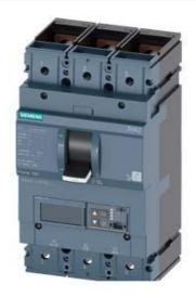
CIRCUIT BREAKER 3VA2 IEC FRAME 630 BREAKING CAPACITY CLASS C ICU=110KA @ 415 V 3-POLE, LINE PROTECTION ETU850, LSI, IN=400A OVERLOAD PROTECTION IR=160A ...400A SHORT CIRCUIT PROTECTION ISD=0,6..10X IN, II=1,5..15X IN NEUTRAL PROTECTION OPTIONAL WITH EXT. CT;UPTO 160% BUSBAR CONNECTION
